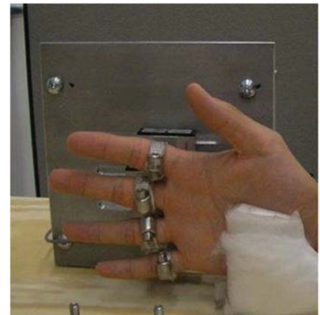
Figure 1. Experimental set up with adjustable plate to set wrist posture. From Sanei & Keir, 2013
